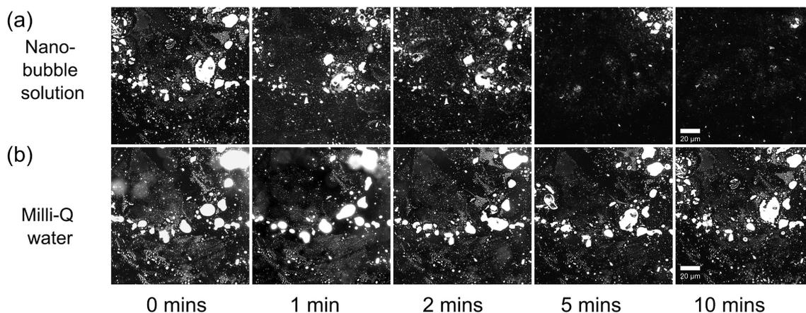
**Figure 7.** Nile blue dyed oil surface-stained glass coverslip under stirring in a) Nanobubble solution after 0 min (start), 1 min, 2 mins, 5 mins, and 10 mins, and a b) Milli-Q solution for 0 min (start), 1 min, 2 mins, 5 mins, and 10 mins. The scale bar is 100  $\mu\text{m}$ .
