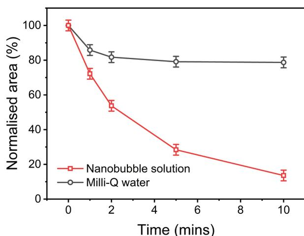
**Figure 8.** Percentage of oil deposits on the glass surface over time. Data was normalized with respect to total fluorescence at 0 min. Wash with Milli-Q water indicated by the black line, wash with the nanobubble solution indicated by the red line.
