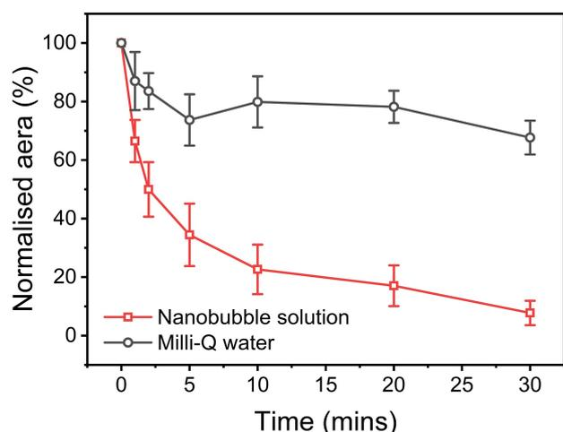
**Figure 10.** Percentage of remaining oil over time. Data normalized with respect to total area of oil at 0 min. The black line represents oil removal using Milli-Q water, and the red line represents oil removal using a nanobubble solution.
