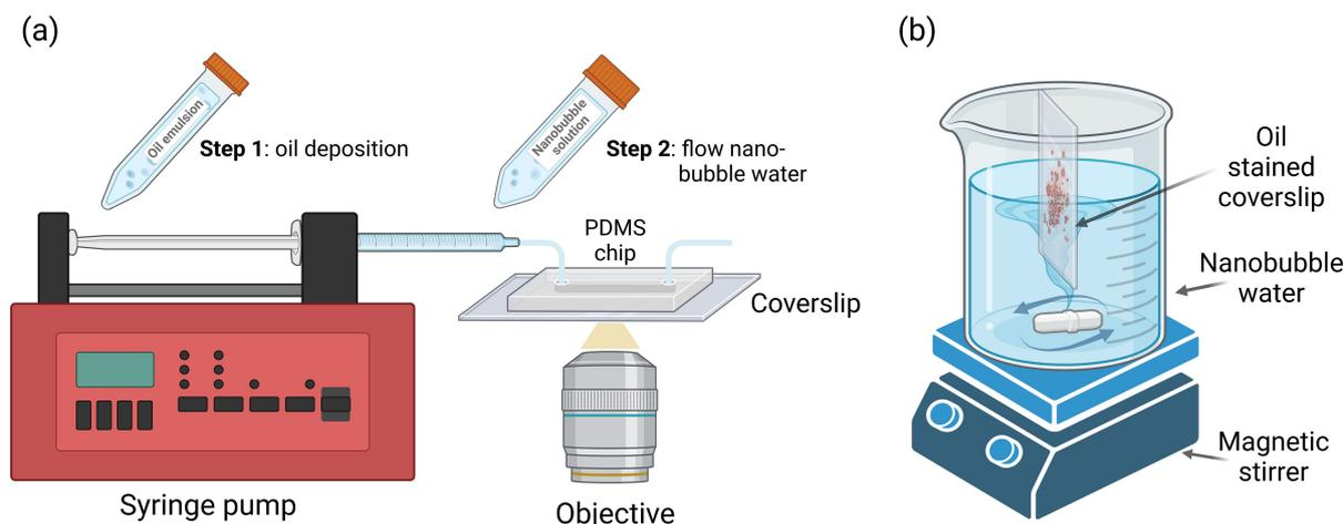
**Figure 1.** Schematic of oil cleaning processes via (a) a microfluidic channel, and (b) mechanical washing. Oil deposition on a glass coverslip was followed by washing with first a control solution without nanobubbles, and then a solution containing nanobubbles. Made with Biorender.com.
