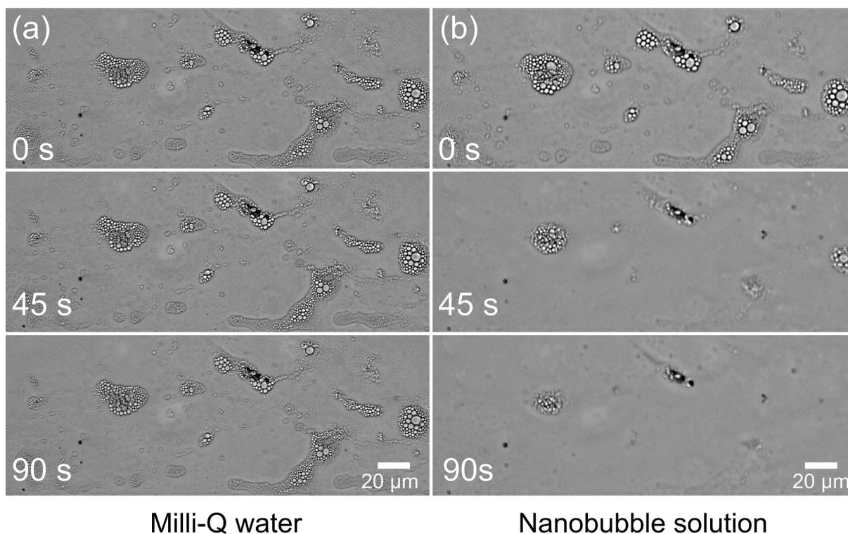
**Figure 3.** Hydrophilic channel with oil deposits washed with Milli-Q water (a) without nanobubbles (control) and (b) with nanobubbles. Representative images taken at 0 s (before introduction to the solution), 45 s and 90 s. The scale bar is 20  $\mu\text{m}$ .
