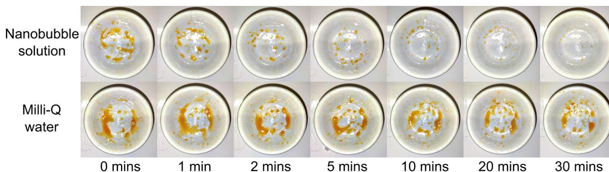
**Figure 9.** Cleaning oil from a porcelain bowl using a nanobubble solution (top) or Milli-Q water (bottom).
