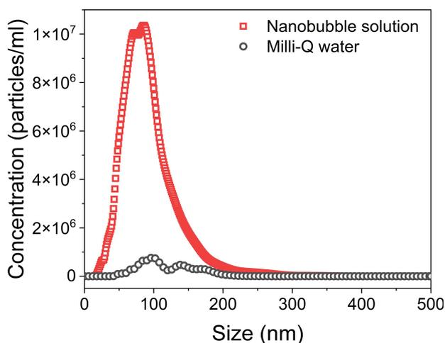
**Figure 2.** The size distribution and particle concentration of the nanobubble solution (red) and Milli-Q water (black) from NTA.
