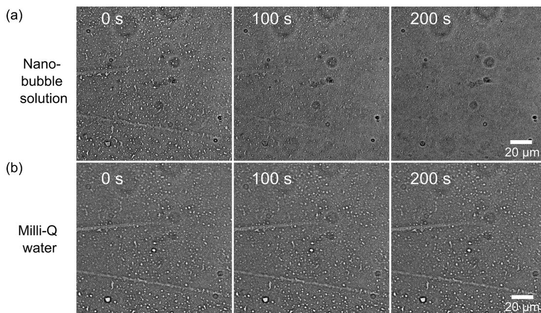
**Figure 5.** Removal of attached oil in a hydrophilic channel using either (a) a nanobubble solution, or (b) Milli-Q water (control). Images taken from a video, with time stamps chosen at 0 s (before introduction to the solution), 100 s, and 200 s.
