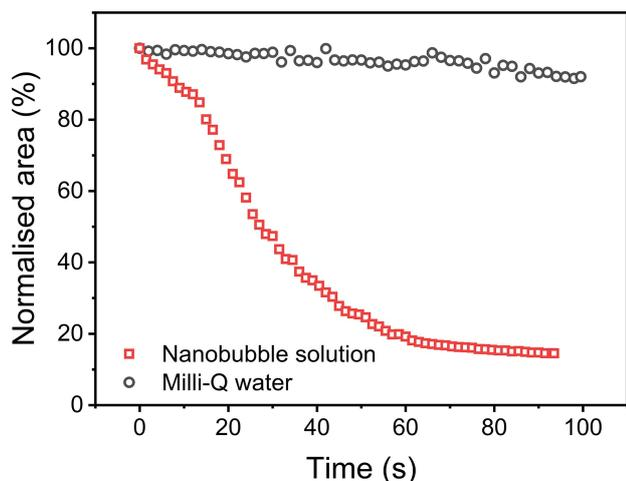
**Figure 4.** Percentage of oil on the hydrophilic surface over time. Data was normalized with respect to total area of oil at 0 s. Wash with Milli-Q water indicated by black circles and wash with the nanobubble solution indicated by red squares.
