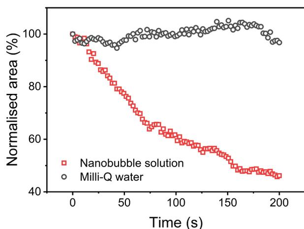
**Figure 6.** Percentage of attached oil on the hydrophobic surface over time. Data was normalized with respect to total area of oil at 0 s. Wash with Milli-Q water indicated by black circles and wash with the nanobubble solution indicated by red squares.
