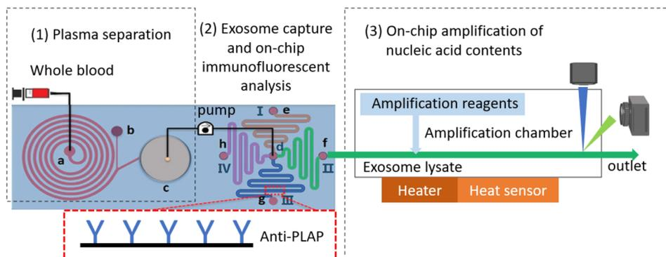
**Figure 6.** A proposed model of fully integrated microfluidic devices for placental exosome isolation, on-chip immunofluorescent analysis, and nucleic acid biomarker detection from whole blood. (1) Plasma separation module, (2) exosome detection module using a specific marker for placental exosome and immunofluorescent analysis, (3) nucleic acid amplification module. Adapted with permission from ref 153. Copyright 2020 American Chemical Society.
