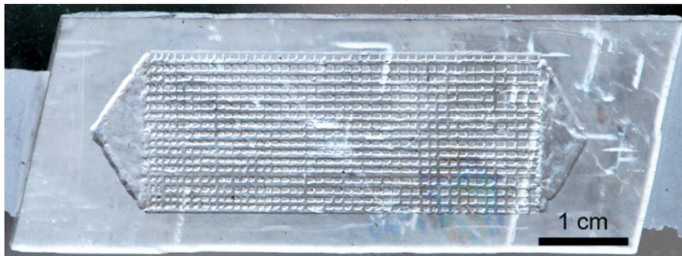
The microfluidic model is etched into a calcite crystal
