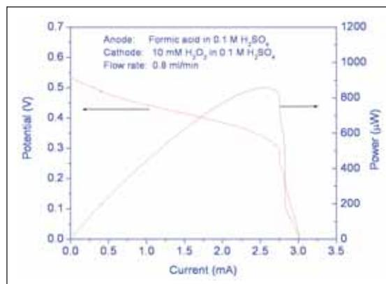
*I-V curve and Power curve of the membrane-less fuel cell. The Fuel stream is 0.5 M formic acid in 0.1 M  $H_2SO_4$  and the oxidant stream is 0.01 M  $H_2O_2$  in 0.1 M  $H_2SO_4$ . The flow rate is 0.8 ml/min*
