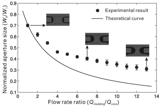
Fig. 2. Relationship between the aperture size (normalized by 1 mm) and the flow rate ratio. The flow rate of the core stream (transparent liquid) is fixed at  $200 \mu\text{l/h}$ , while the flow rate of the cladding stream (black ink) is variable from 200 to  $2600 \mu\text{l/h}$ .
