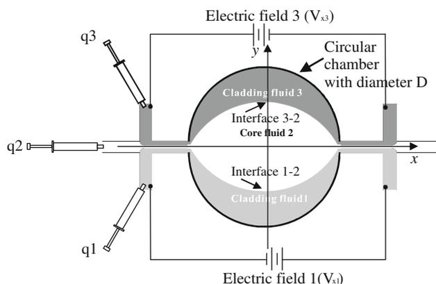
**Fig. 1** Schematic representation of the optofluidics lens under the combined effect of hydrodynamic and electroosmosis
