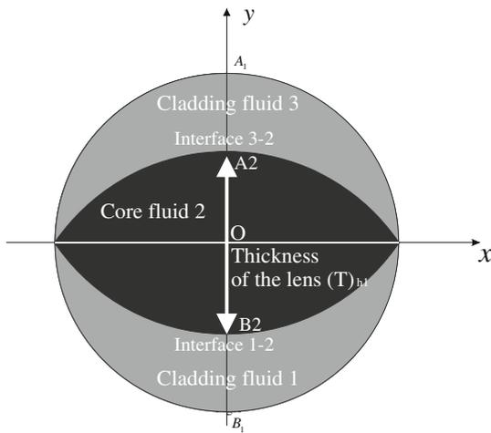
**Fig. 4** The interface positions of a lens
