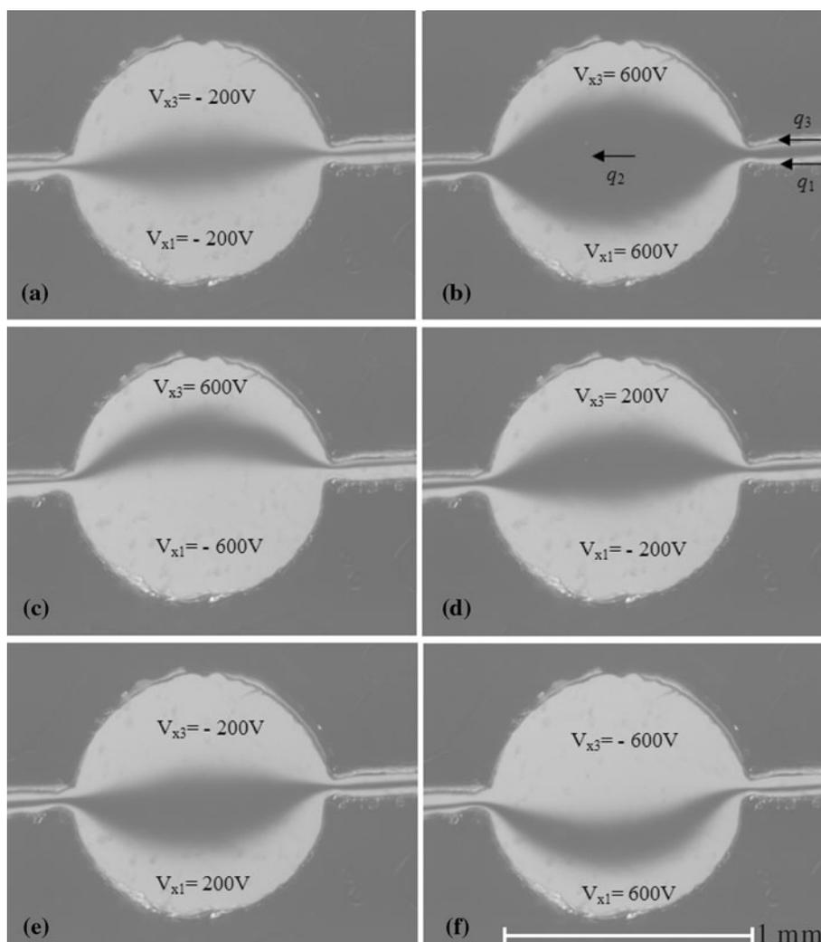
Figure 8 shows a series of different optofluidic lenses. The electroosmotic effect for controlling optofluidics lens is confirmed experimentally. Figure 8a–f shows that at a fixed flow rate, the curvatures of the interfaces (interfaces 1–2 and 3–2) can be modified according to the magnitudes and the polarities of the voltages.
