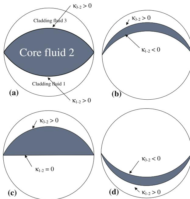
**Fig. 5** The definition of the symbol of curvature and the model of lens. The core fluid is regarded as a region. Convex region has  $\kappa > 0$ , concave region has  $\kappa < 0$ , and a plan has  $\kappa = 0$ . **a** Biconvex lens; **b** meniscus lens; **c** plano-convex lens; **d** meniscus lens
