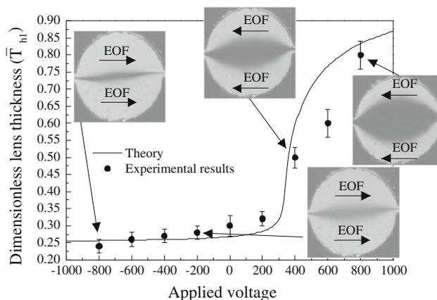
**Fig. 9** Thickness of the lens verse applied voltage ( $q_1 = q_2 = q_3 = 0.05$  ml/h,  $L_{ref} = 1$  mm,  $V_{x1} = V_{x3}$ )
